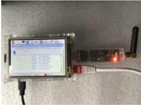
*Left: a DV4Mini being used with a Raspberry PI computer. I like this approach as it avoids tying up a PC (important if you have family!), as well as requiring less power and being easy to 'put out of harm's way'. It can be located anywhere within WI-FI range or be connected via wired Ethernet. It supports multiple digital modes and incorporates a low power 70cm transceiver (10mW max power output). Choose a quiet frequency within 70cm in your area – no NOV required.*
